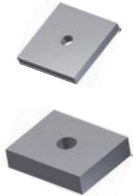
Flat Plates are used for timber or steel walings in conjunction with a winged nut or a hex nut for load transfer. The embossing of the plate increases its rigidity. Load capacity depends on the contact area, the admissible bearing pressure and the threadbar that is used.
