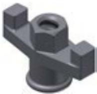
With different Waler Plates, Wing Nuts can be used as anchor nuts both for timber and steel walings. They can be fixed and loosened using a hexagon wrench or a threadbar. If necessary, a clamping effect can be attained or overcome by applying hammer strokes to the wings.
